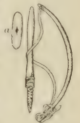
BOW DRILL WITH STONE POINT. a, HAND-PIECE
